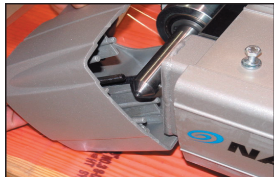
Figure 8.3: Installing alignment bolts
